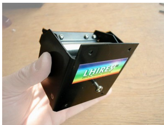
Grating holder can be switched very quickly on a Lhire III spectrograph
